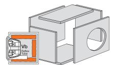
**Damping material:** FONOFORM on all the inside walls except for the speaker's.
